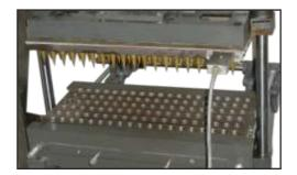
The ZE 50-PN series of semi-automatic machines are used for baking ice cream cones, moulded sugar cone and cups. These machines are easy to use and robust. The heating is by electrical heaters designed to optimize energy use and thermal distribution; This machine is flexible for high production on nonstop basis for 24 hours.
